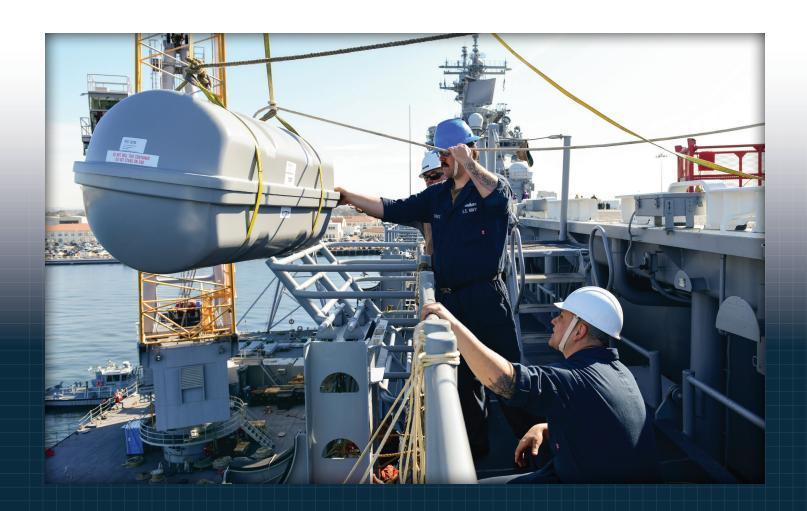
Underway, Boxer sports 116 life rafts in case of emergency. Every five years, these rafts are removed for inspection and re-packing and then re-installed. With the help of a crane, several safety harnesses, and skilled line handling, the deck department spent a day installing 50 rafts off the starboard side of the ship.
